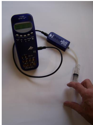
Fig. 1: Measuring the absolute pressure in relation to the volume
