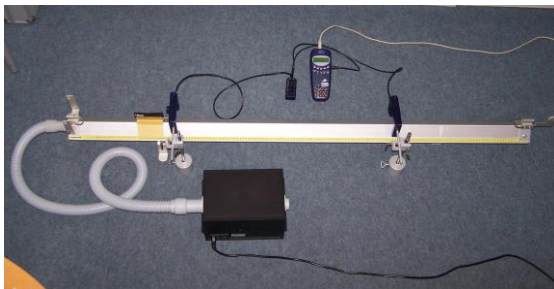
Fig. 1: Measuring the velocity of a glider over a given distance on the air track
