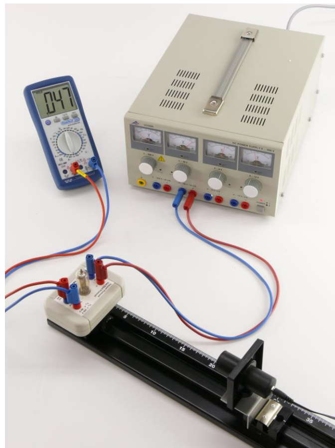
Fig. 2 Experiment set-up for demonstrating the photoelectric effect
