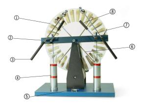
The Wimshurst machine serves as a source of safe, high DC potentials for numerous experiments in the area of electrostatics.
