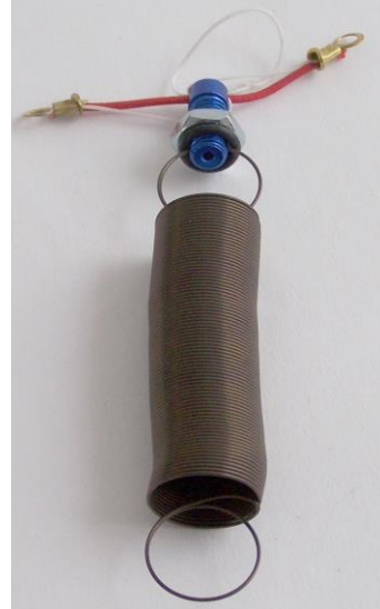
Fig. 2 Spring module with coil spring
