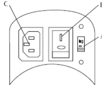
Fig. 1 A voltage selector switch, B power switch, C socket
