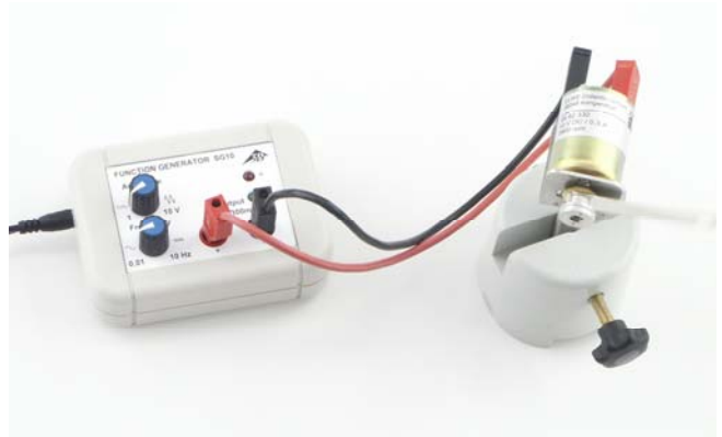
Fig. 1 Experiment set-up for demonstration of rotation reversal for a DC motor
