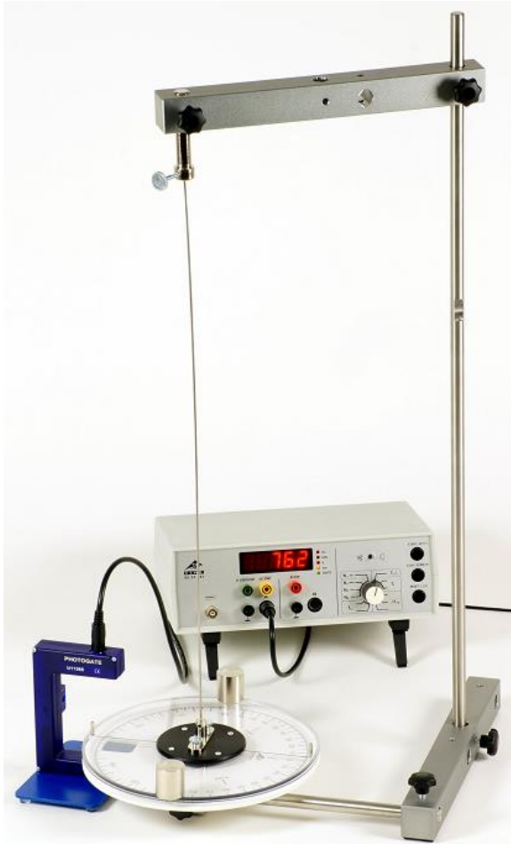
Fig. 10: Dynamic measurement using light barrier and digital counter.
