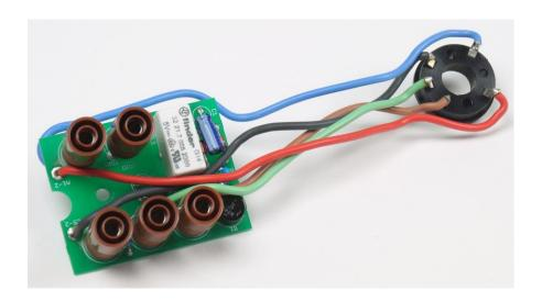
The quality of the electron beam in electron deflection tube S (1013889) is affected by the resistance between sockets C5 (cathode) and F4 (heating filament) on the tube. For optimum results, the resistance  $R_{\text{C5F4}}$  needs to be 390 k $\Omega$ . Tube holder S (1014525) is accordingly designed such that this resistance is present.
