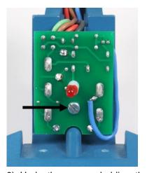
8) Undo the screws holding the printed circuit board. Be careful, because the screw is inside a spacer ring, which you must not lose.
