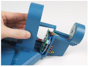
3) Carefully pull the guide pillar up at an angle, making sure that the LED is not damaged.
