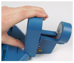
2) Place your thumb under the guide pillar at the bottom, using this as a fulcrum. Gently pull the bar to lever the base out of the tube holder.
