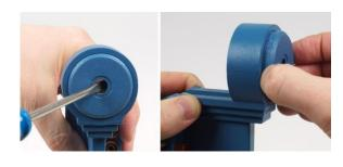
5) Carefully lever the cap out a little way using a screwdriver and then take it out the rest of the way with your hand.
