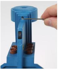
4) Use the hex key to undo the hex screw on the base of the tube holder.
