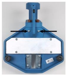
1) Turn the tube holder over and undo all the screws.
