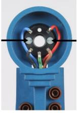
6) Undo the screws for the contact ring.
