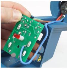
9) Carefully pull the board forwards and lift the terminal sockets out of their guides.
