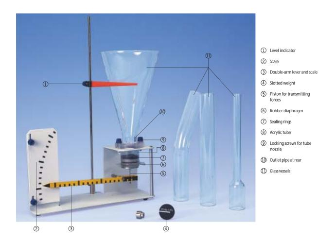
Pascal's vane apparatus is used for demonstrating the hydrostatic paradox and for quantitative measurements of pressure at the bottom of a fluid column as a function of its height.
