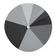
The colour disc is used to prove that an additive mixing of individual colours of the visible spectrum results in the colour white.
