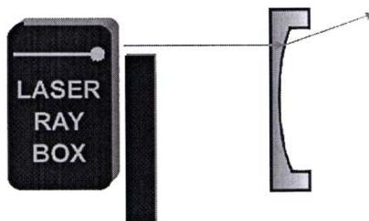
**E15b Light beam passing through convex glass-air boundary**
