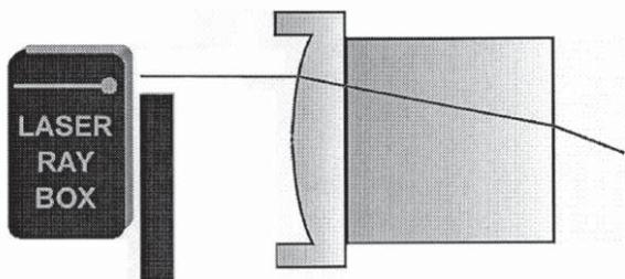
**E13b Light beam passing through convex air-glass boundary**
