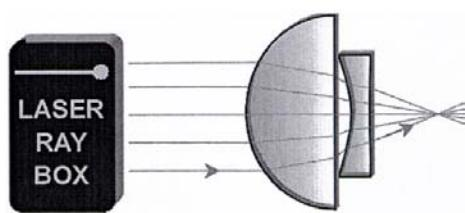
The figure is created by parallel rays, so it is unreal and magnified. If the top ray of the incident beam is obscured, the top ray of the output beam disappears.
