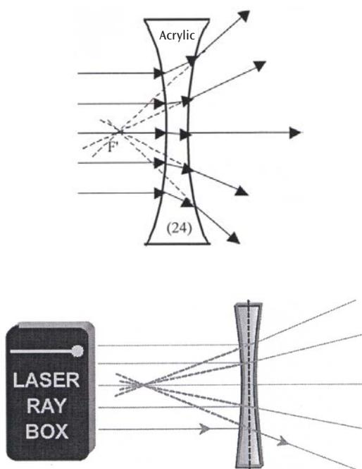
**E18b Light beam passing through glass concave lens – the rays are non-parallel to the optical axis**
