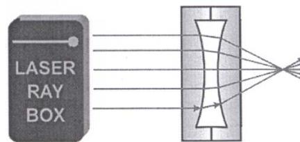
**E20b Light beam passing through air concave lens – the rays are non-parallel to the optical axis (U17301)**
