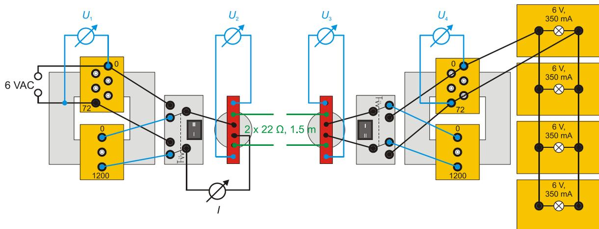
**d) Model of transmission line with high line resistance using stepped-up voltage**
