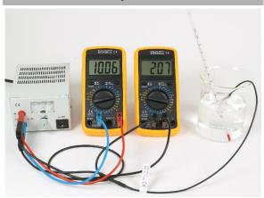
Measure the current at 10 V DC as a function of the temperature of the water bath, and calculate the resistance from this.
