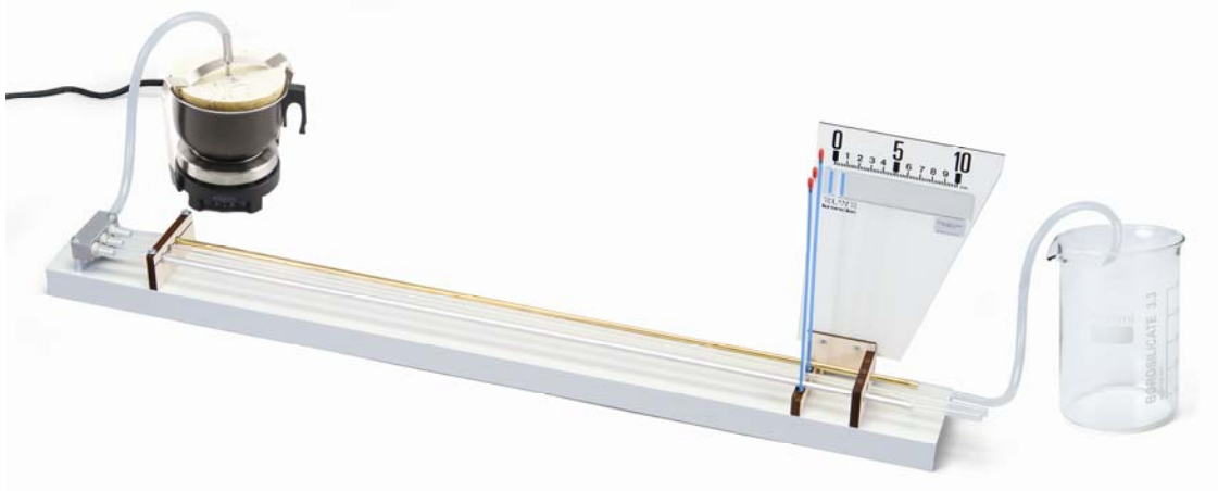
Fig.1 Experimental set-up with the linear expansion apparatus, dilatometer (U8442200)
