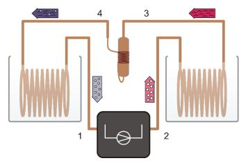
Fig. 2: Schematic representation of the heat pump with a compressor (1, 2), condenser (2, 3), expansion valve (3, 4) and evaporator (4, 1)
