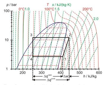
Fig. 3: Representation of ideal cyclical process for heat pump in a Mollier diagram
