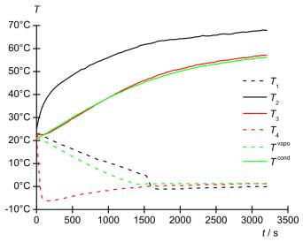
Fig. 4: Changes in temperatures  $T_1$ ,  $T_2$ ,  $T_3$ , and  $T_4$ , over time at measuring points 1 to 4 and  $T^{\text{vapo}}$  and  $T^{\text{cond}}$  for the cold-water and hot-water reservoirs respectively. Black: compressor, red: expansion valve, green: water reservoirs. Solid lines: hot side, dotted lines: cold side
