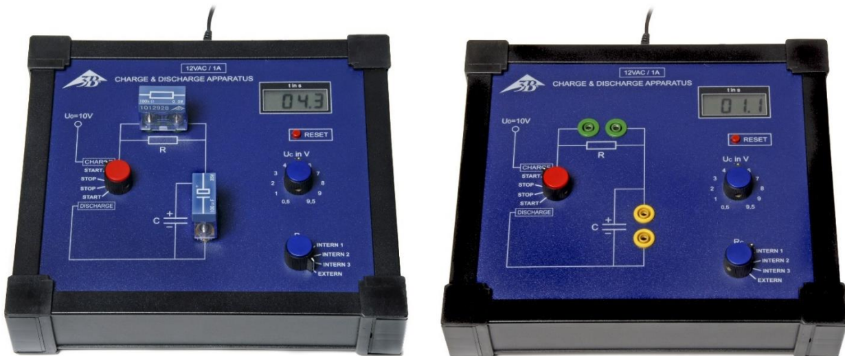
Fig. 1: Charge/discharge equipment in operation with external (left) and internal (right) resistor/capacitor pair.
