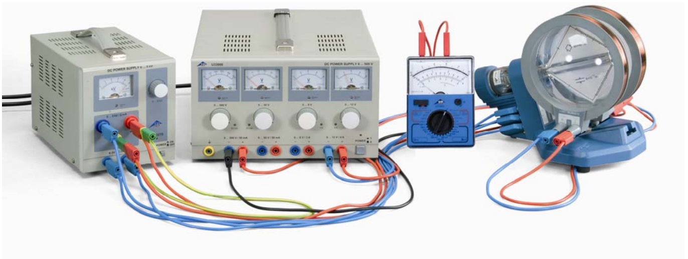
Fig. 2: Experiment set-up for investigating deflection of electrons by magnetic and electric fields.
